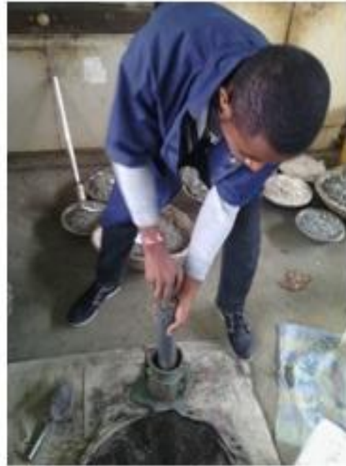
Fig. 7: Picture showing compaction Test
