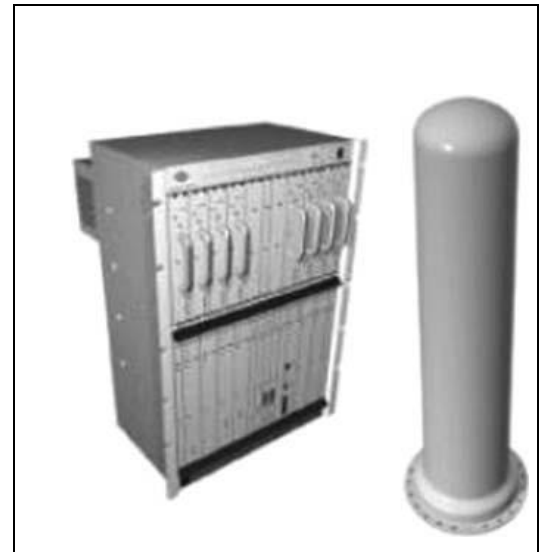
Figure 1.2: WiMAX base station.
