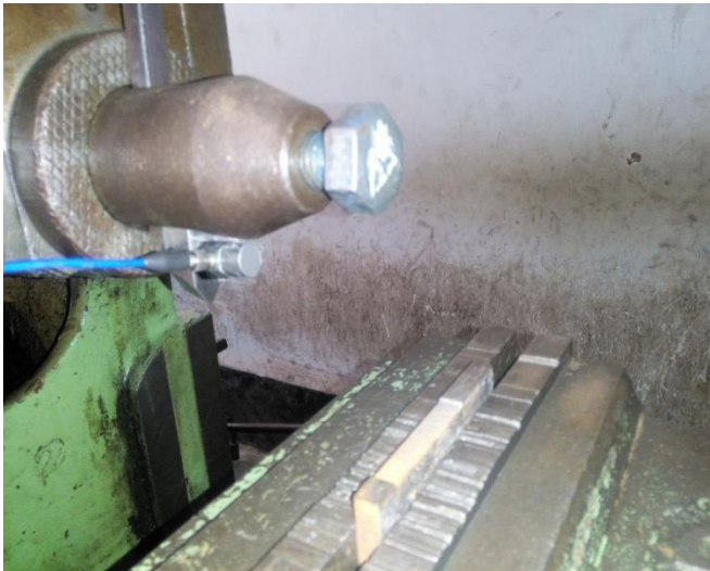
Fig -2: Accelerometer mounted on the tool during working of machining
