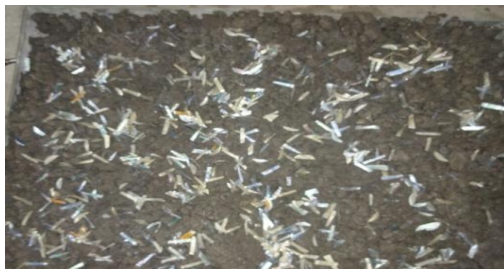
Fig- 2 Bottle cap fibers added to concrete
