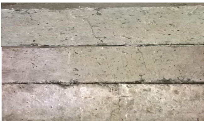
Fig. 6 Crack pattern and failure mode of beam without fibre
