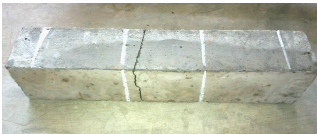
Fig. 6 Crack pattern and failure mode of beam without fibre
