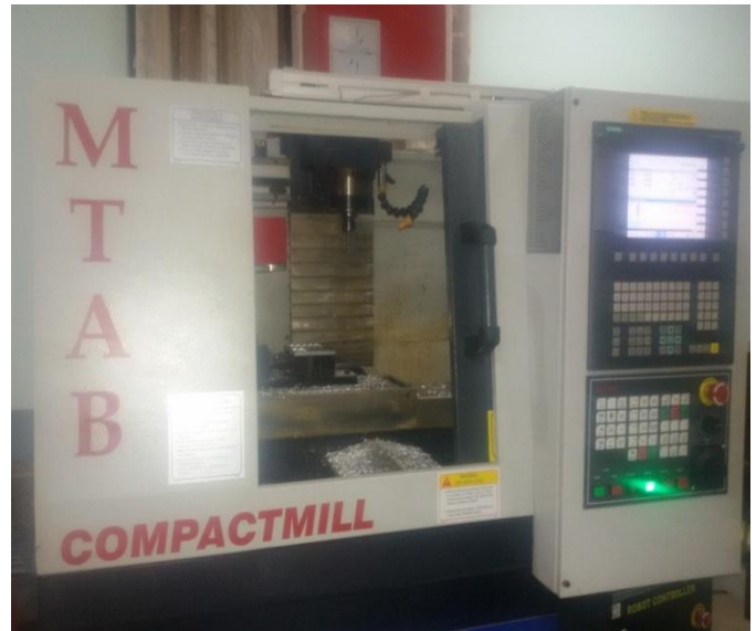
Fig.1.Experimental set up for end milling
