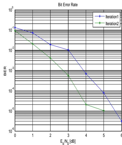
Fig 5 BER plot for log-map decoder: Punctured [4]
