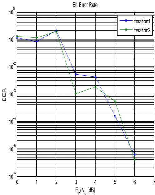
Fig 7 BER plot for SOVA decoder: Punctured
