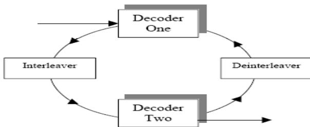
Fig.2 Turbo decoder [2]
