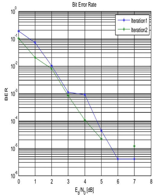
Fig 8 BER plot for SOVA decoder: Unpunctured [5]
