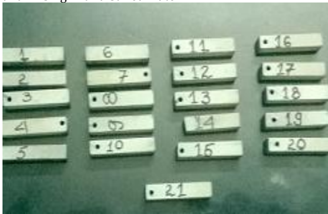
Fig-1: Specimen's detail (MAO coating on Al Alloy) The specimen Chemical Composition test was done at M/S Indiana Ferro Alloys, Mohali according to ASTM E1231-2011 as shown in Table 1.
