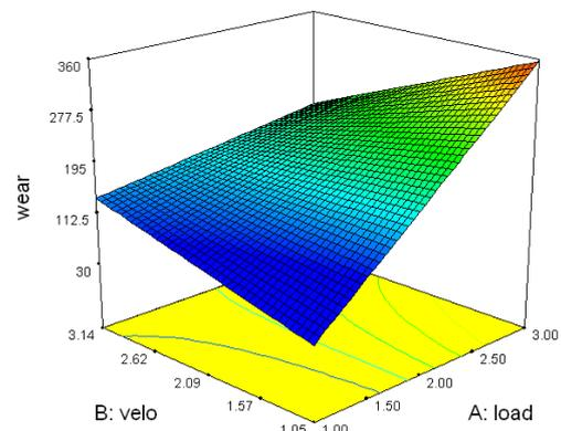
Fig 5 Interaction effect of load and velocity on wear for Al-Im25 +SiC
