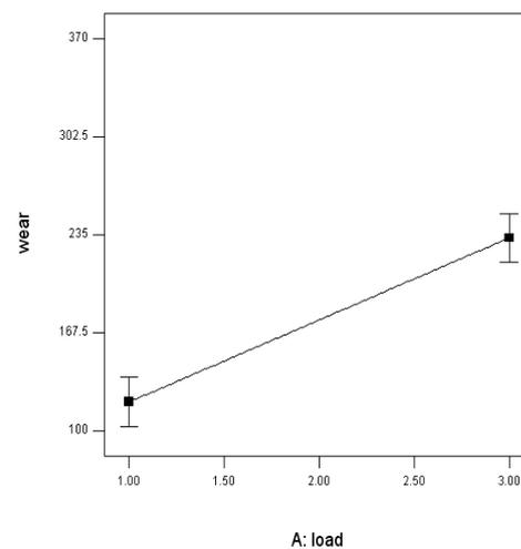
Fig.3 (a)- Wear v/s load for Al-Im25+10%SiC
