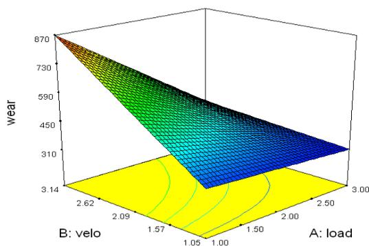
Fig.4- Interaction effect for velocity and load on wear for Al-Im25
