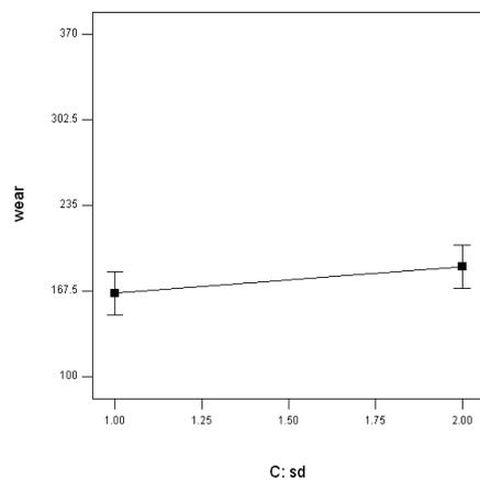
Fig.3(c) Wear v/s sd. for Al-Im25+10%SiC
