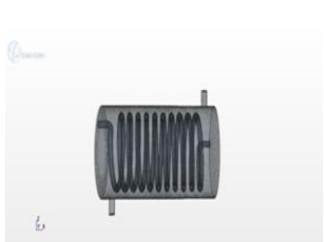
Fig 2: Designed model of heat exchanger.
