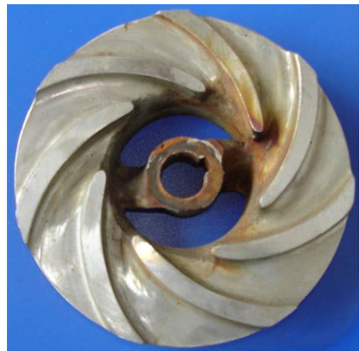
Fig 1. Impeller after trimming to final diameter
