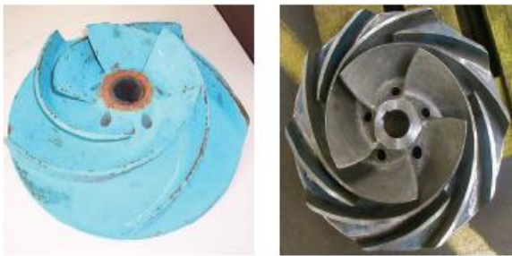
Fig 8. Original (left) and splitter (right) impellers.
