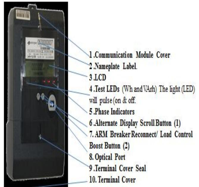
Fig -1: Smart meters with components explained . AMI three phase meter start with 0530xxxxxx. Unauthorized access and safety of customer and personnel indicated separately.
