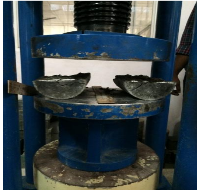
Fig-4 Split tensile strength test
