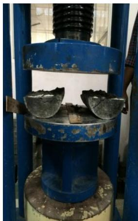
Fig -4 Split tensile strength test
