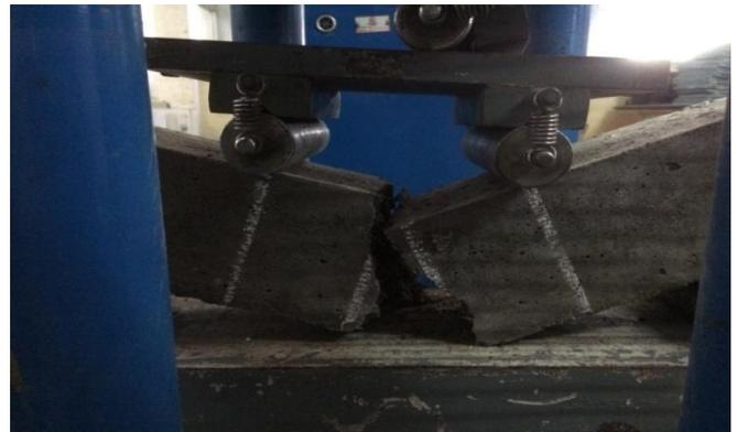
Fig -5 Flexural strength test
