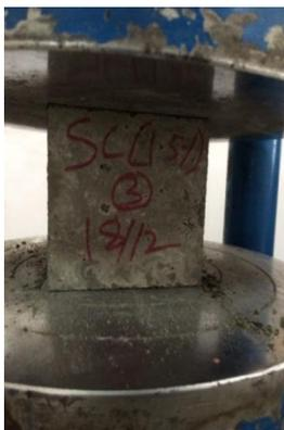
Fig -3 compressive strength test
