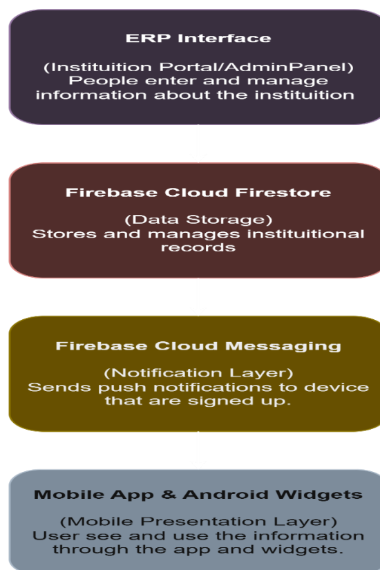
Figure 5: Data flow of the intelligent ERP System
