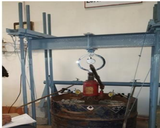
Plate - 6: Experimental Cyclic Plate Load Set for Finding Load - Settlement
