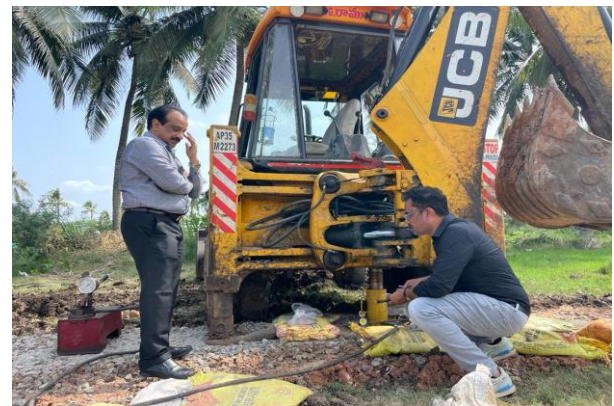
Plate - 8: Authors conducting field load test on Prepared Test track
