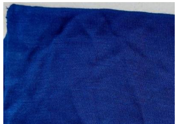
Figure 21 (100% viscose knitted fabric with strips or barre defect)
