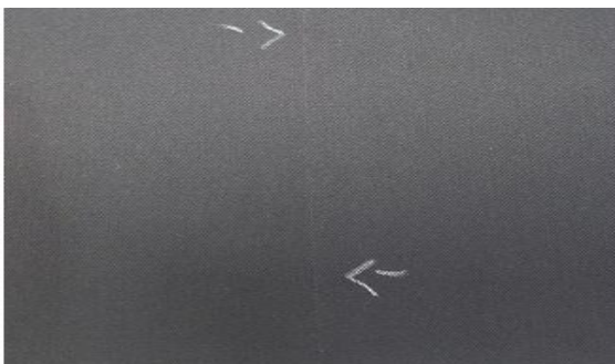
Figure 10 (Woven fabric with a white line barre)
