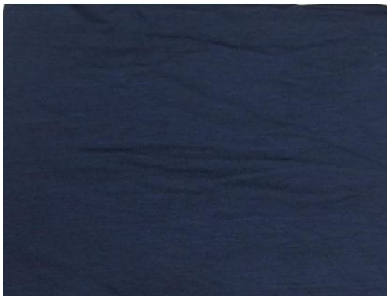
Figure 19 (100% viscose knitted fabric with periodic light line or barre)
