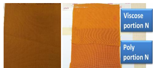
Figure 14 (Woven fabric with warp wise streaks/barre)
