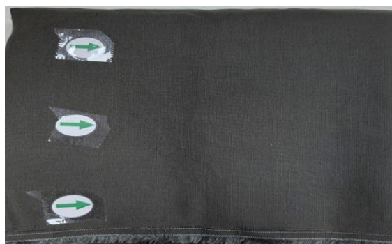
Figure 23 (Woven fabric with barre in warp yarn)
