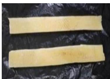
Fig. (6a) HDT Test Samples
