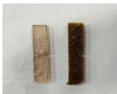
Fig 3 a:- Izod Impact sample after notching
