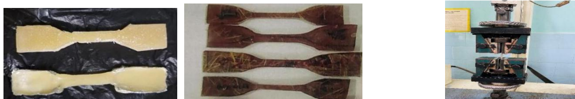
Fig.: 2a Tensile sample of epoxy Fig :-2b Tensile sample of 10 % wood + epoxy Fig: 2c Tensile testing
