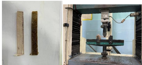
Fig (4 a):-Samples for Flexural property determination
