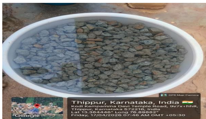
Fig 2 Soaking of demolished concrete
