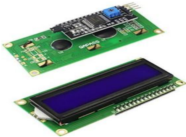
Figure 5 LCD Display with IO expansion
