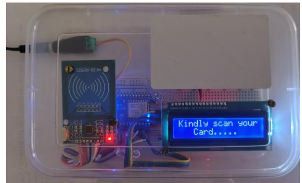
Figure 9 Place the RFID tag in RFID reader module
