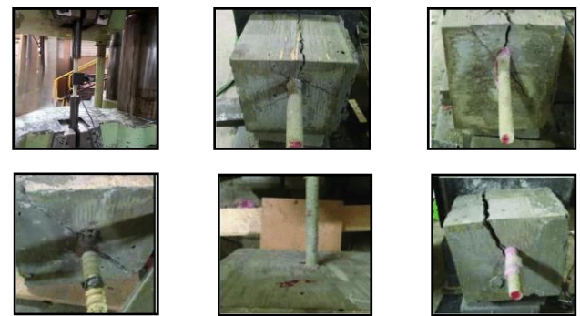
Fig -3: Bond Strength Test (Pull-Out Test) for Steel Bar
