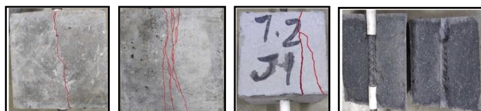
Fig -2: Split Tensile Strength Test on Concrete (M30 mix)
