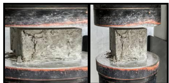
Fig -1: Compressive Strength Test on concrete - (M30 mix)
