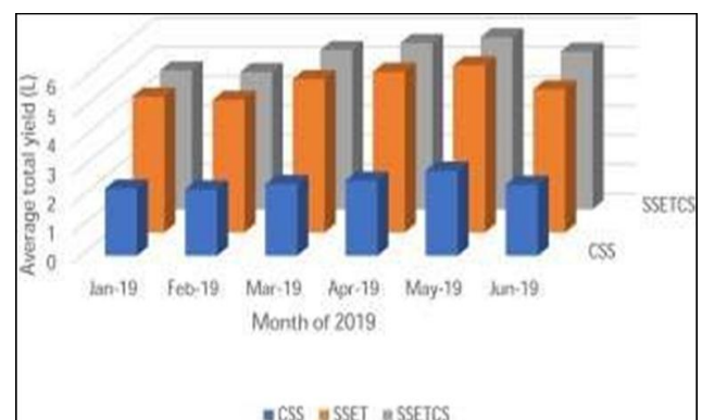
Figure 6: Average total yield from the conventional solar still, solar still with evacuated tubes, and solar still with evacuated tubes and calcium stones between January and June 2019 (22).
