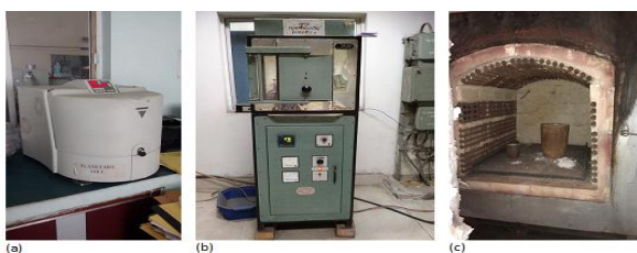
Figure 2.3 (a) Planetary mill used for wet balling of HAP for more fine size, (b) Programmable furnace and (c) Therelek furnace used in FSHAP synthesis.
