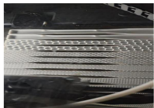
Fig11: Infilled specimens being printer
