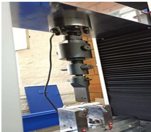
Fig15: Universal Flexural testing
