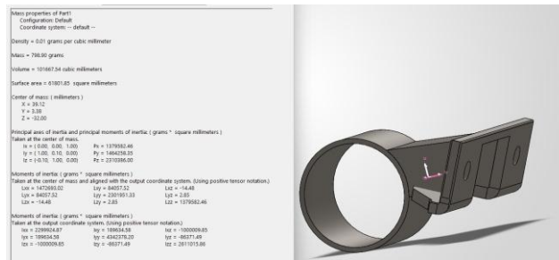
Fig 3: CAD cross section and mass properties
