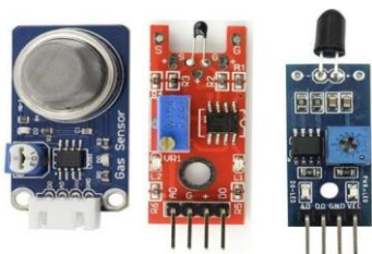
Fig. 1: MQ-2 Smoke Sensor, LM35 Temperature Sensor, and IR Flame Sensor
