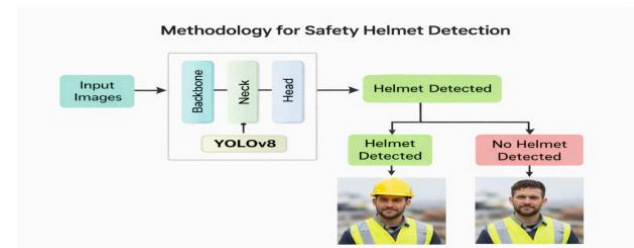
Fig -1: Methodology for Safety Helmet Detection
