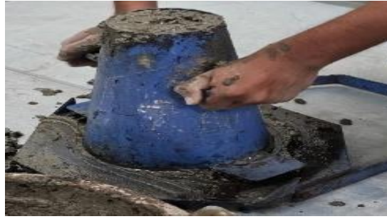
Fig 6. Slump Cone Apparatus
