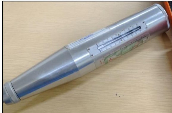
Fig 9. Rebound Number testing Apparatus
