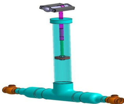
Figure 2.3: Perspective View of the oscillating cylinder, piston, reciprocating connecting rod and paddle foot rest subassembly.
