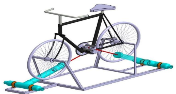
Figure 3.1: Perspective view of assembly of pedal operated oscillating cylinder reciprocating pump in accordance with a preferred embodiment of the present invention.
