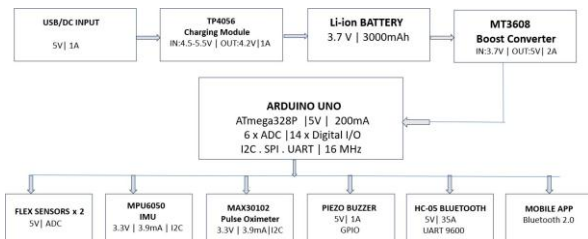
Fig. 1. Detailed Block Diagram of the smart glove system
