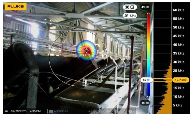
Figure 1.4: Snapshot from the AHS BC-01 acoustic report showing Section 172 roller 1 with measured level 45 dB
