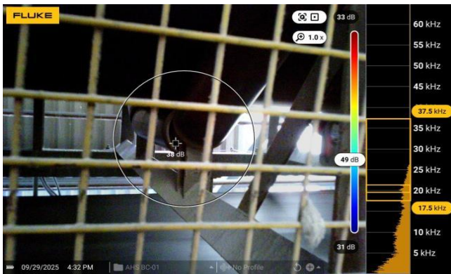
Figure 1.3: Snapshot from the AHS BC-01 acoustic report showing Section 184 roller 1 with measured level 38 dB
