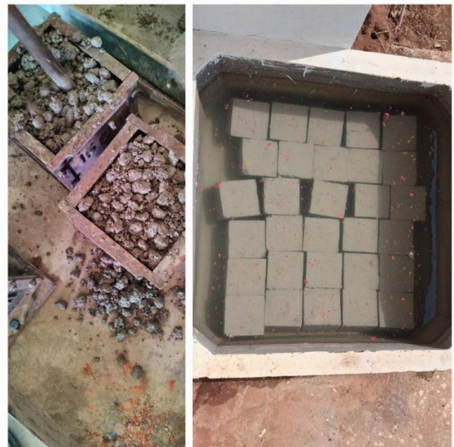
Fig -2: Casting and Curing of cubes
