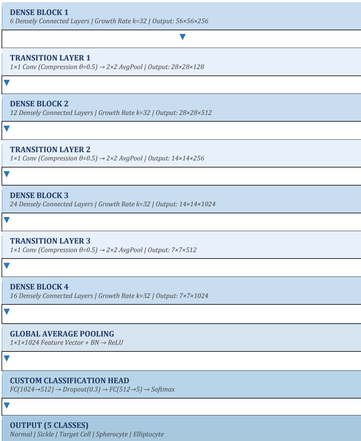
Figure 4: End-to-end DenseNet-121 pipeline for RBC morphology classification. Each Dense Block implements H_l(x) = \text{BN-ReLU-Conv}(1 \times 1)\text{-BN-ReLU-Conv}(3 \times 3) bottleneck operations. Growth rate k=32 governs the number of feature maps added per layer. The custom classification head replaces the original ImageNet 1000-class output with a 5-class Softmax layer.
