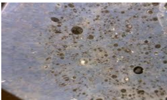
Fig.3. Image of Blow hole defect
