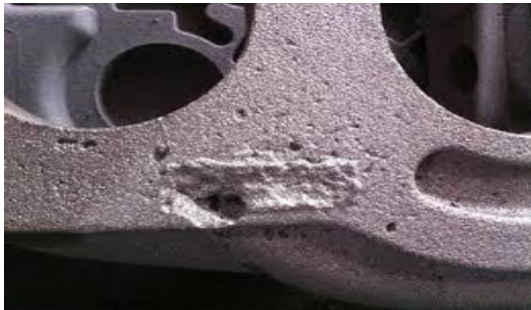
Fig 7. Image of Rubbing defect
