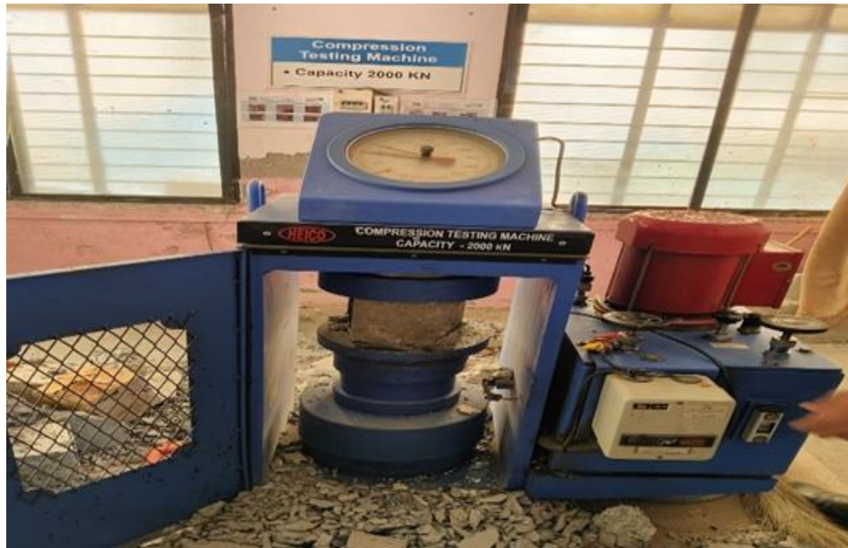
Figure 3: Compressive Strength Cube Test
