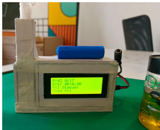
Fig-2: Physical Prototype of Oil Sense in action, showing the LCD displaying R, G, B, and GR values with the 'Used Oil' status.
