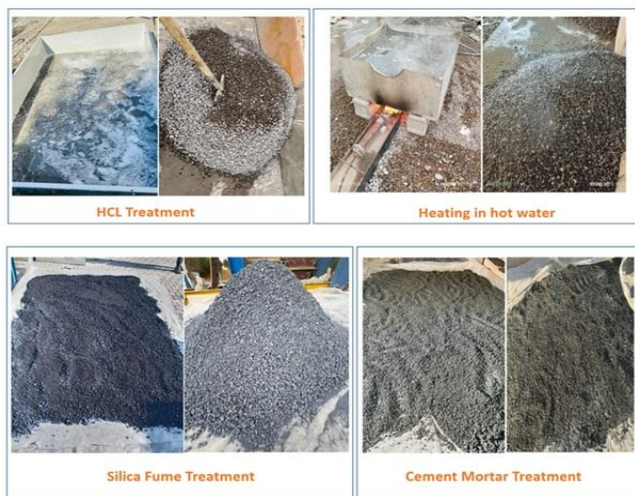
Fig -3: Treatment methods of RCA
