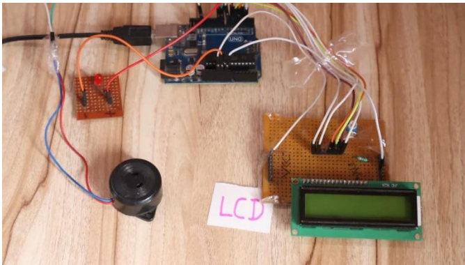
Fig -1: Embedded hardware setup featuring Arduino Uno and active buzzer.
