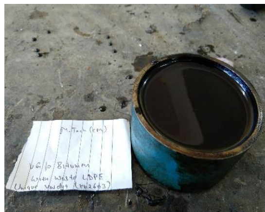
Figure 4.2:-Sample for Penetration Test
