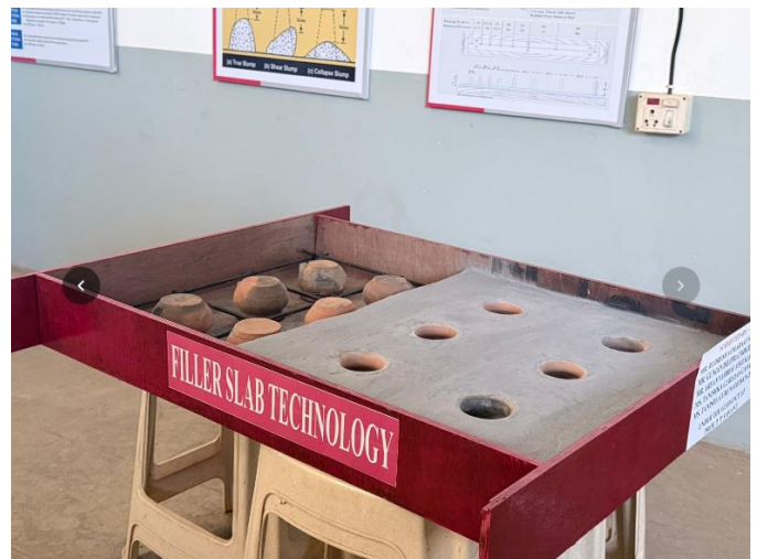
Fig -4: Filler Slab
