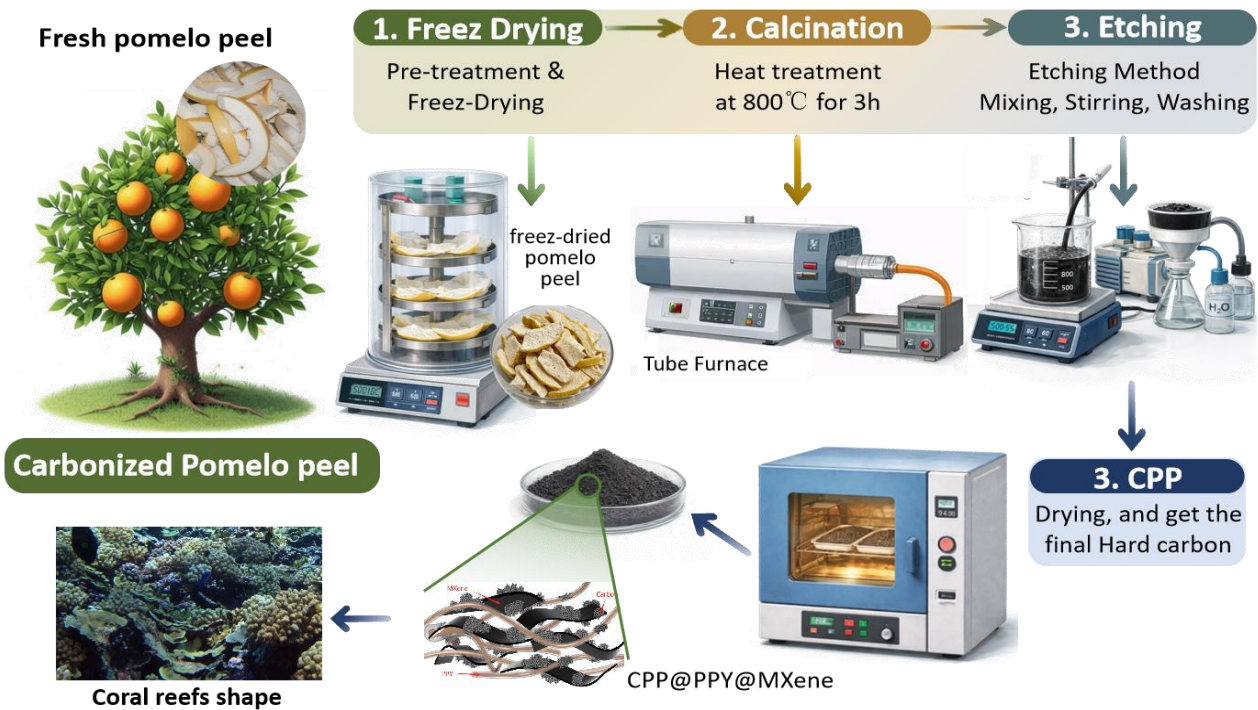
Fig- 1: schematically present the circle to get the main formula CPP@PPy@MXene passing by the Carbon activation and Mxene preparation to get the wanting formula.
