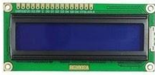
Fig. 8. 20×4 character LCD with PCF8574T I 2 C backpack at address 0x27. Three-screen rotation: temperature and humidity (3 s), rainfall status and gas level (3 s), atmospheric pressure (1 s). Alert messages override rotation immediately.
