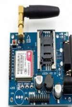
Fig. 7. SIM900A GSM modem module. UART serial interface; GSM 900/1800 MHz. Replacement whip antenna (right) required for stable network registration — original stub antenna maintained insufficient signal margin.
