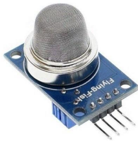
Fig. 5. MQ-series gas and smoke sensor module. Heated tin-dioxide sensing surface; 12-bit ADC input on GPIO 34. Potentiometer configures digital trigger threshold; analogue output used in firmware. Dual-read confirmation and 45-second warm-up suppression implemented.
