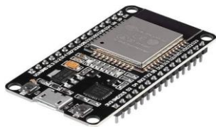
Fig. 2. ESP32-WROOM-32 microcontroller development board. Dual-core 240 MHz Xtensa LX6 CPU; 520 KB SRAM; 4 MB flash; integrated 802.11 b/g/n Wi-Fi; 18-channel 12-bit ADC; 36 usable GPIO.
