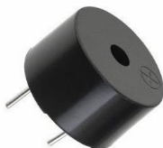
Fig. 9. Active piezo buzzer on GPIO 27. Two 500 ms pulses per alert event; audible at 8 m through closed corridor. Active buzzer type requires DC voltage drive only — no transistor driver needed at 30 mA.
