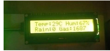
Fig. 12. 20×4 LCD during normal operation. Temperature 29 °C, humidity 67 %, rain status 0, gas ADC 1687 — all parameters within safe threshold boundaries. Three-screen rotation active.
