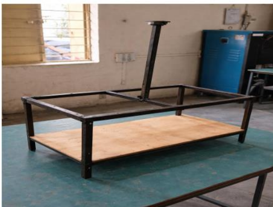
6. Vertical Shaft / Pipe The pipe holds the wind turbine at a suitable height for wind flow.
