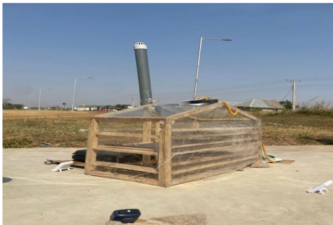
Fig -3: Greenhouse solar dryer during experiment
