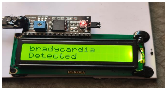
Fig -5: LCD Display Showing Bradycardia
