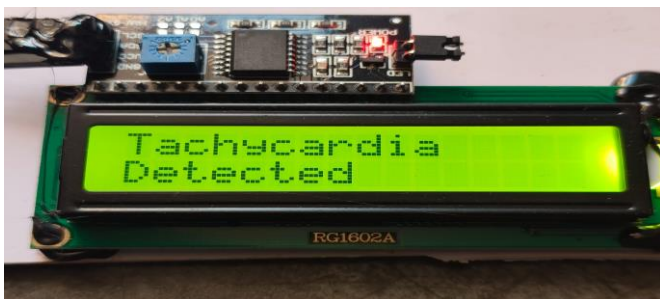
Fig -4: LCD Display Showing Tachycardia
