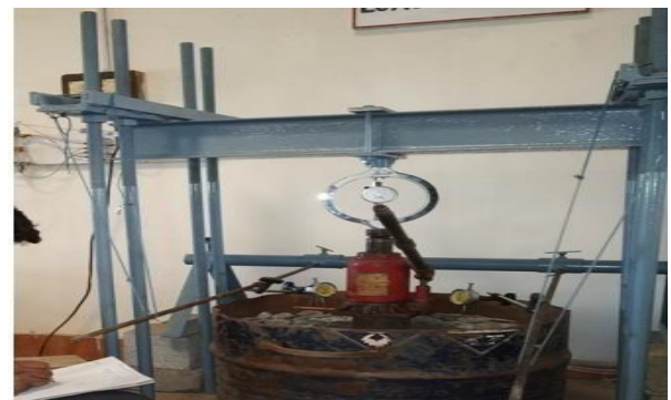
Fig - 4: Experimental Cyclic Plate Load Set for Finding Load – Settlement
