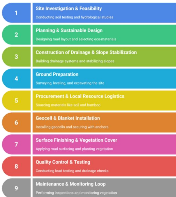
Figure 3: Construction process of geocell road
