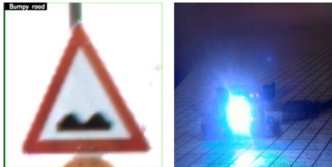
Fig - 14 : Detection sign : Bumpy road + bounding box + Blue light indication + sound
