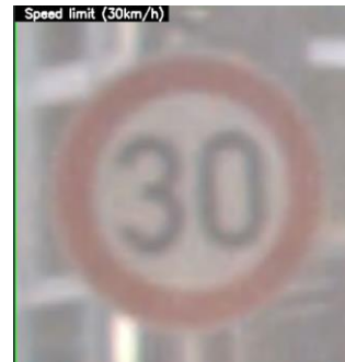
Fig - 10 : Detection sign : Speed limit(30km/h) + bounding box + Red light indication + Sound
