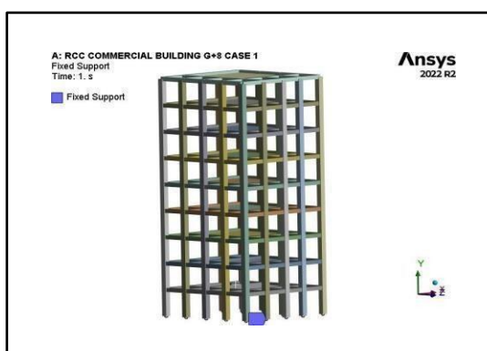
Fig: 5 Fixed Support of G+8 Building.
