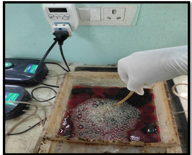
Fig.2.2: (a) Diffuser performance testing
